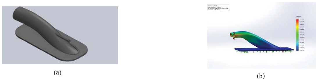
Fig.7. (a) 3d design of jet propulsion unit (b) Simulation of jet propulsion unit
